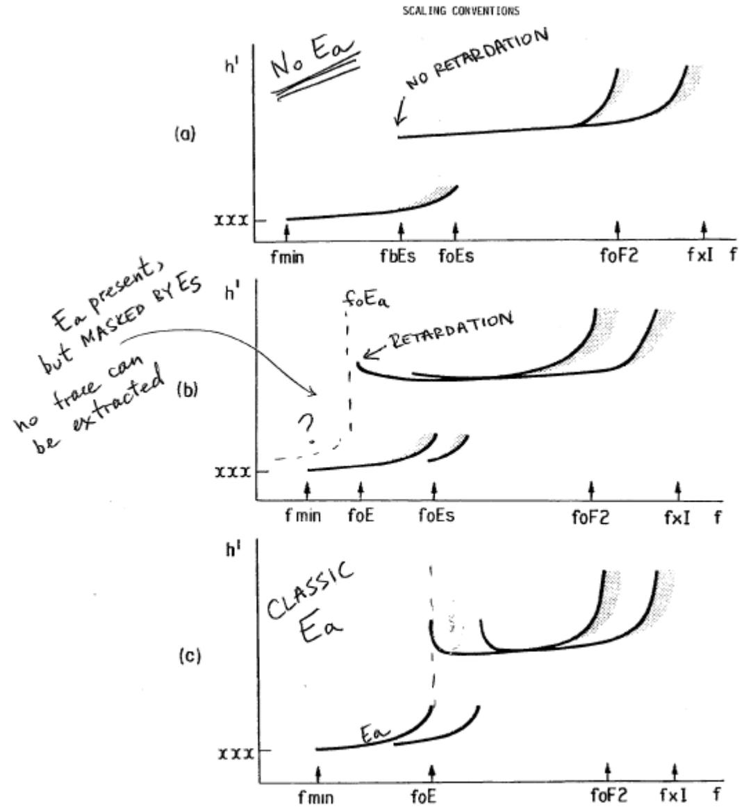
Fig. 4.2 Conventions for Es type r and particle E
